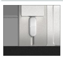
The guiding channel can assist with the tablet orientation to ensure correct measuring position.
