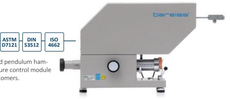
Fully-automatic digital measuring device with guided pendulum hammer, external electronic unit and optional temperature control module for the determination of rebound resilience on elastomers.
