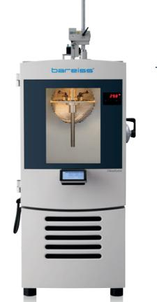
High-quality temperature control or climatic chamber in conjunction with the proven hardness tester digi test II, rotation table and software with database function, for serial testing of the hardness of polymers according to Shore A, D or IRHD N, depending on the temperature.
